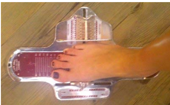
Fig. 1, Standard Brannock device used for accurately measuring foot lengths and widths
